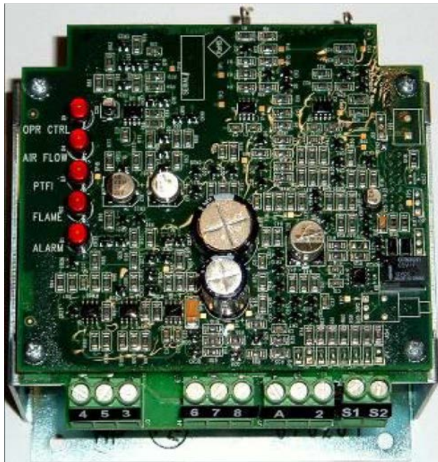
Figure 19 - Flame Safety Controller
